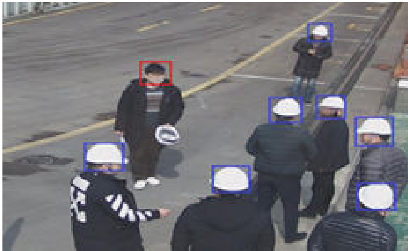
Figure 3-10 Safety helmet and reflective clothing detection
